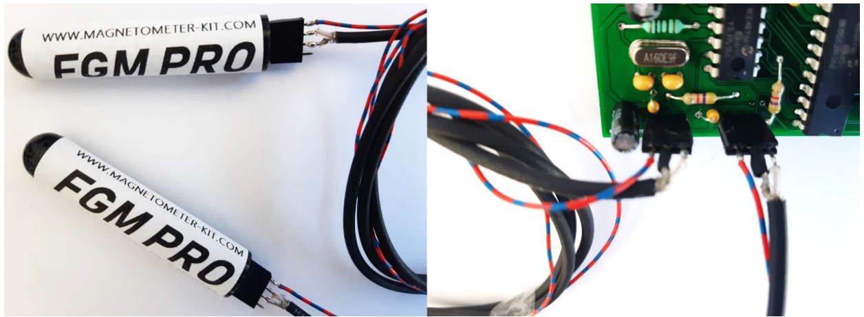
Connector orientation from PCB to sensor
